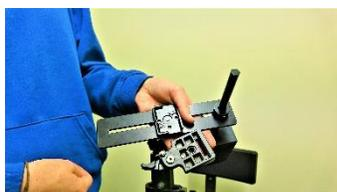
4. Open the Lever Catch to release the QR base from the QR plate. Note the relationship between base and plate.
