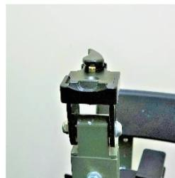
7. This shows the final position of the QR base when fitted. You will need a 9/16"-15mm spanner. It needs to be tight!
