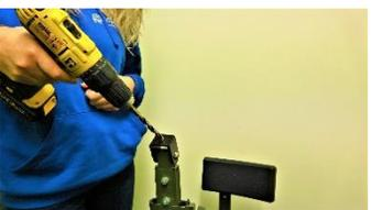
2. Enlarge the hole in the top of the bracket to 9.5-10mm. De-burr the hole.
