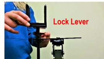
11. Slacken the Lock Lever to enable you to open the jaws of the gun cradle. See Cradle Adjustment above.
