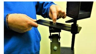
10. The direction on the cradle is best set when sat on the chair with the rifle, to suit l/h r/h and shooting style for your comfort. Lock in place with the screw as shown.
