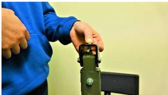
5. Insert the 3/8" bolt through the hole in the bracket so the threads are pointing upwards.
