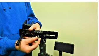
3. Unscrew the 3/8" bolt from the underside of the quick release base
