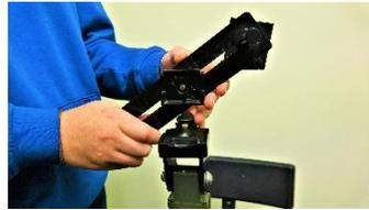
8. With the Lever Catch on the QR base pointing outward – insert the QR plate into the base. The Lever will automatically close.
